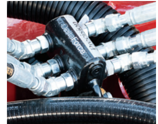
DeltaForce row unit down pressure control
